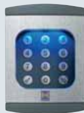
Radio code switch FCT 10b The radio code switch FCT 10b offers the following additional functions in contrast to the code switches CTR 1b and CTR 3b: simple installation, since no cables need to be routed, with up to 10 radio codes (868.3 MHz) for actuating up to 10 doors.
